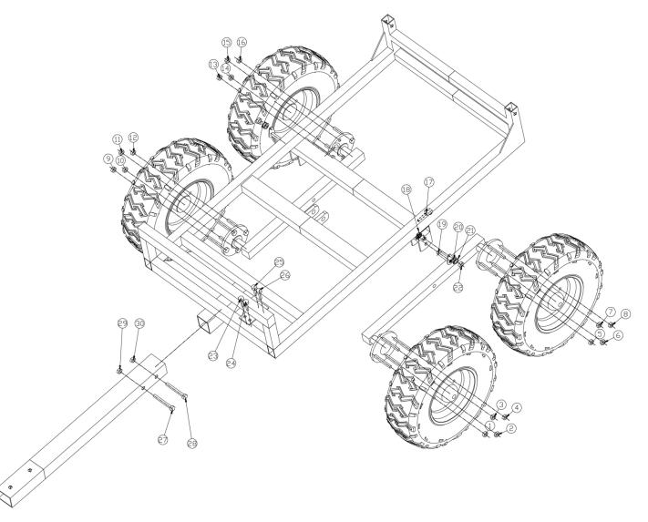
2. Install the net frame &the jack, then install the stanchion, using 2-M16\*50 bolt, M6 nut. Tighten the nut after adjusting to the appropriate position. Install the linear, using Ø12\*70bolt M12 nut, install the capacity seat plate with 4-Ø8\* 20 bolt, M8 nut, Install the tool box with 2 -Ø6\*20 bolt, M6 nut. SEE FIGURE 2.
